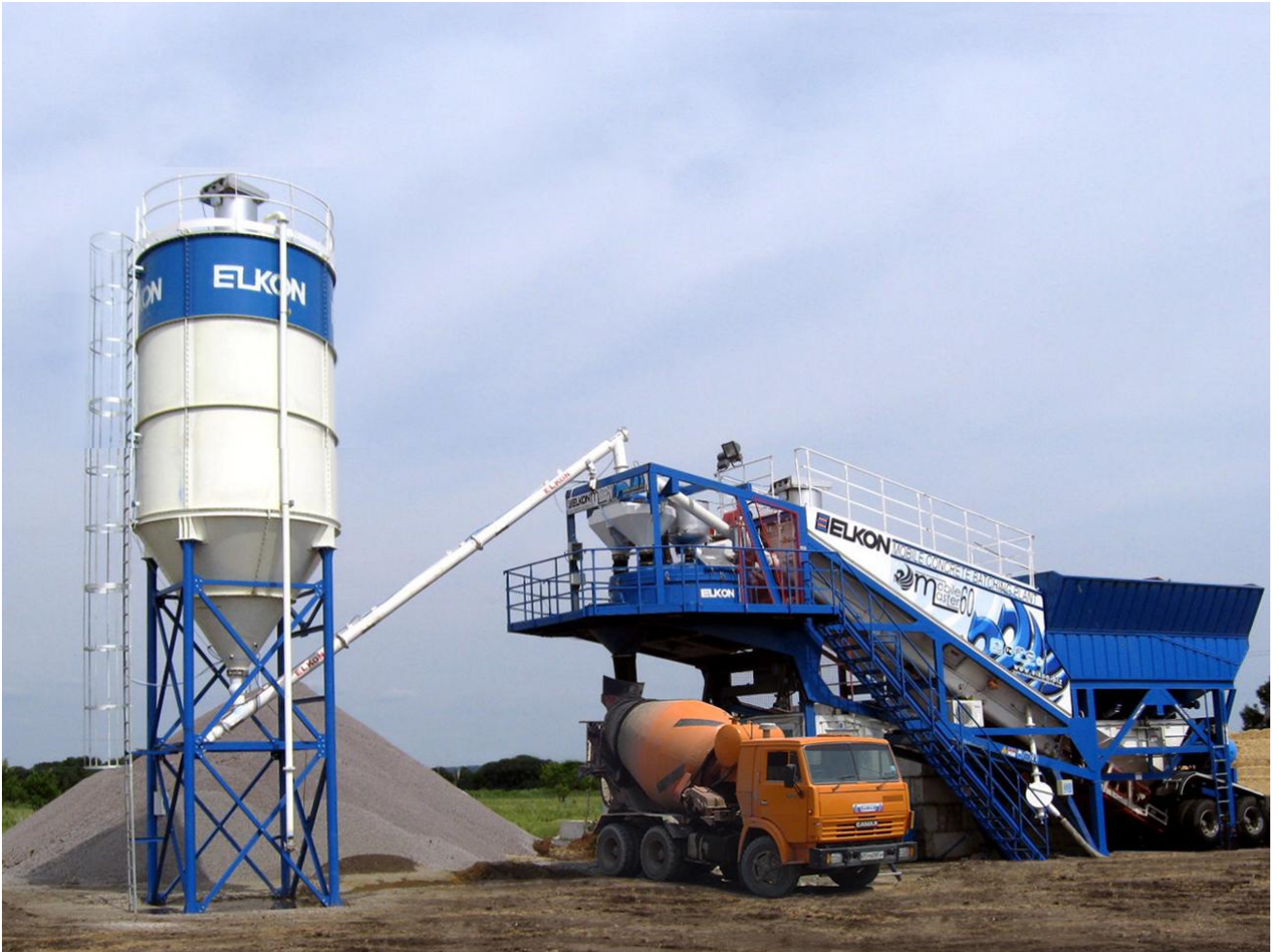
Working Position of ELKON MOBILE MASTER-60 Fully Automatic Mobile Concrete Batching Plant
