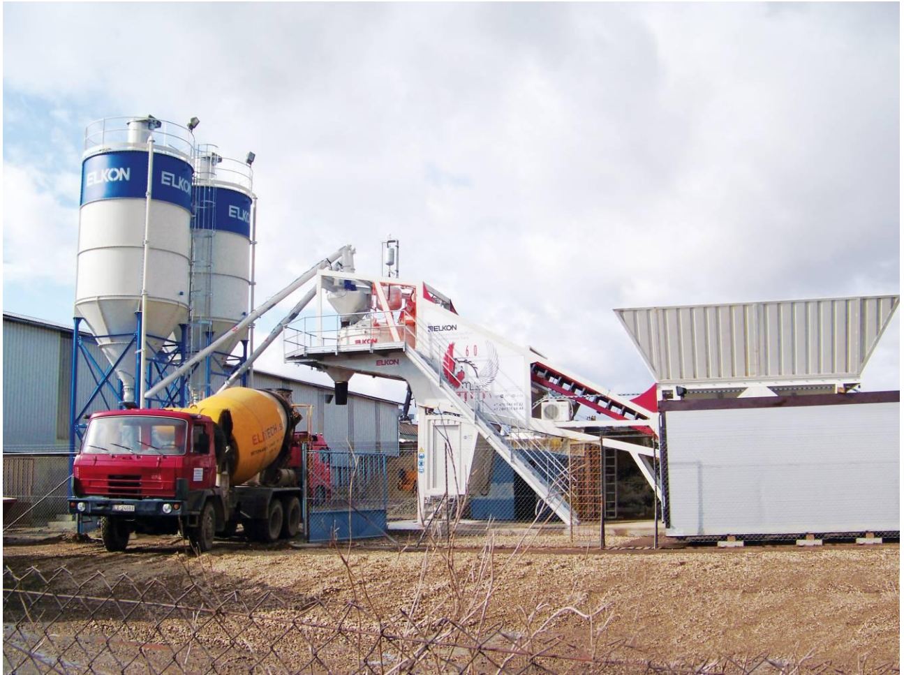
Working Position of ELKON MOBILE MASTER-60 PEGASUS Fully Automatic Mobile Concrete Batching Plant
