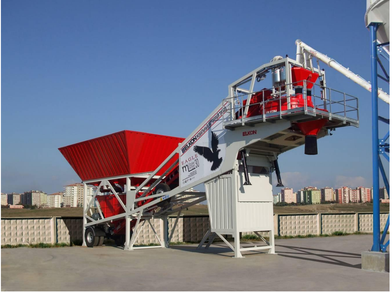
Working Position of ELKON MOBILE MASTER-30 EAGLE Fully Automatic Mobile Concrete Batching Plant with 50 tons cement silo
